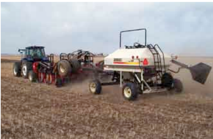
An example of an air drill with disc openers seeding native grasses at Swift Current, Sask.
