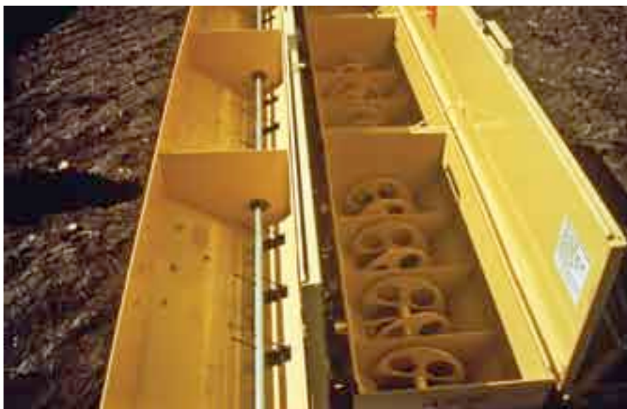
Agitators ensure an even flow of native grass seeds from the drill box to the furrow opener.
