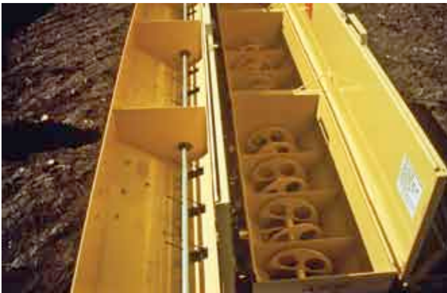
Agitators ensure an even flow of native grass seeds from the drill box to the furrow opener.
