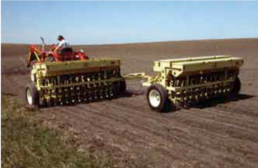
All units in a multi-drill hitch must be calibrated to ensure accurate seeding rates.
