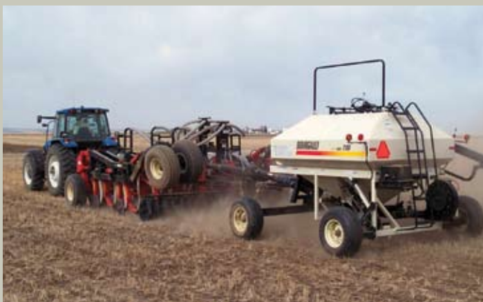
An example of an air drill with disc openers seeding native grasses at Swift Current, Sask.
