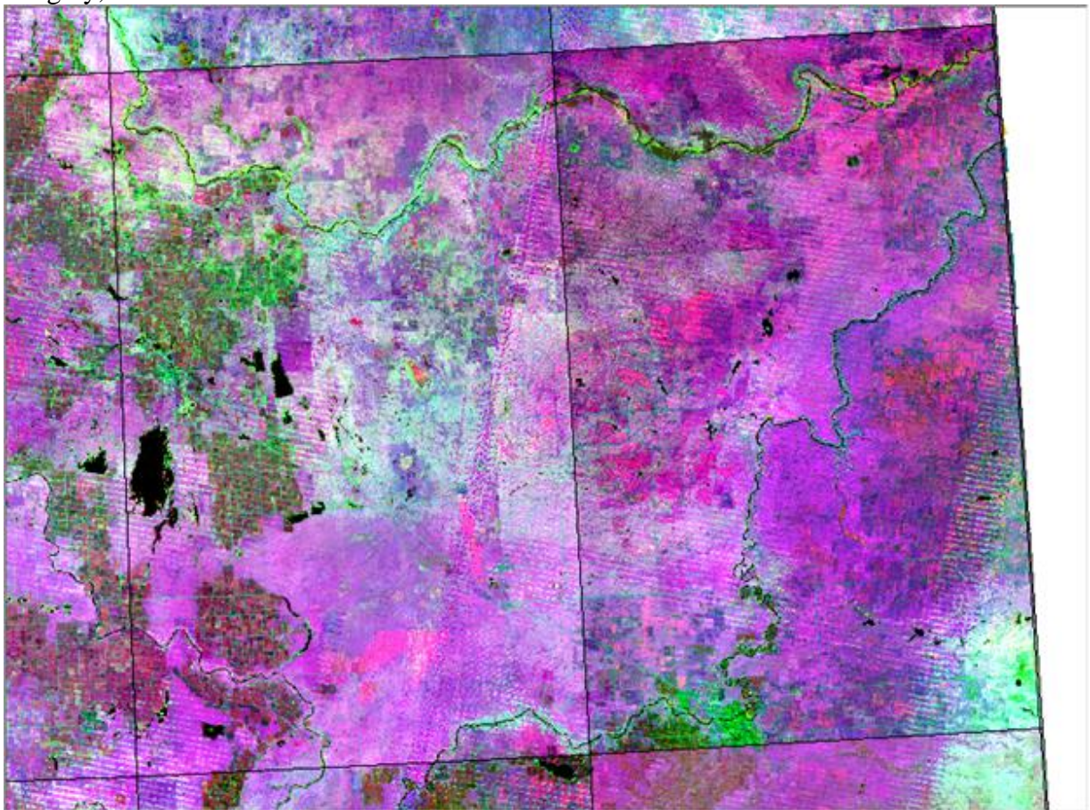
Figure 28. Example of Striping effect in the Timescan products derived from LandSAT 7 imagery,
